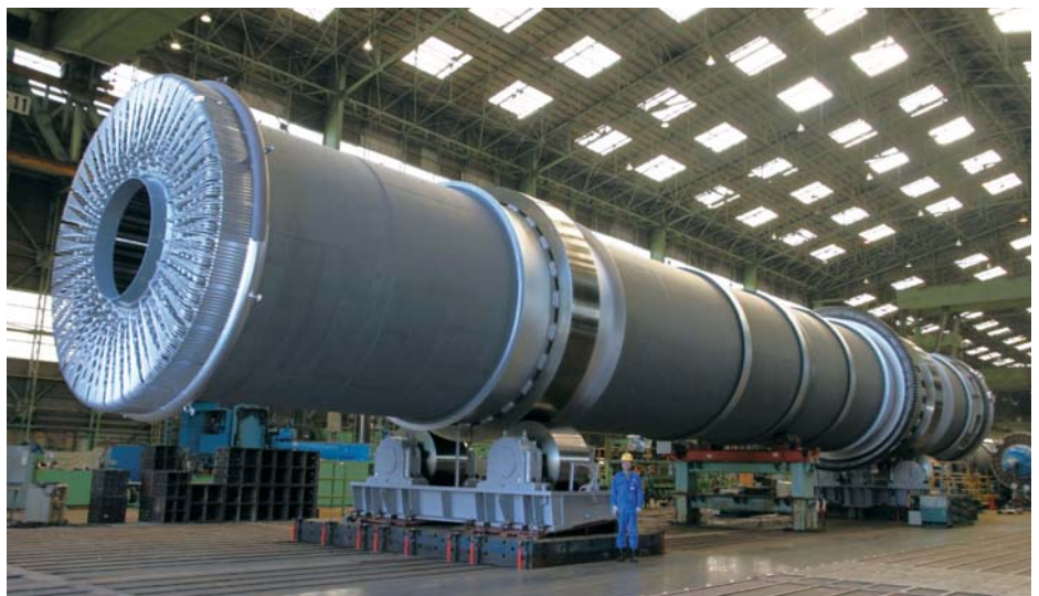
Steam tube dryer
